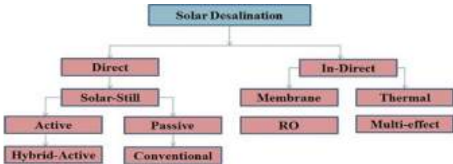
Fig. 1. Classification of solar desalination on the basis of direct and indirect solar energy utilization.
