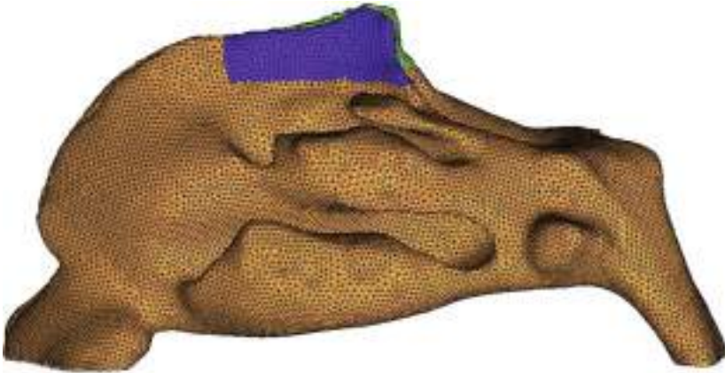
Fig. 2. Computational mesh model of nasal upper airways
