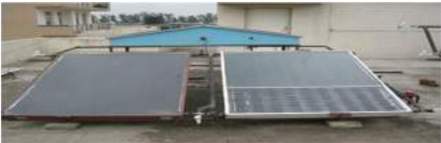
Fig. 2. Hybrid active solar still, Double slope PVT hybrid active solar still [11]
