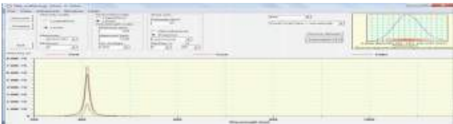
Fig. 2. MIE scattering, silver in glass ( C_{ext}/C_{sca}/C_{abs} Vs wavelength)
