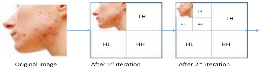
Fig. 1. Two level image decomposition using 2-D wavelet transform.
