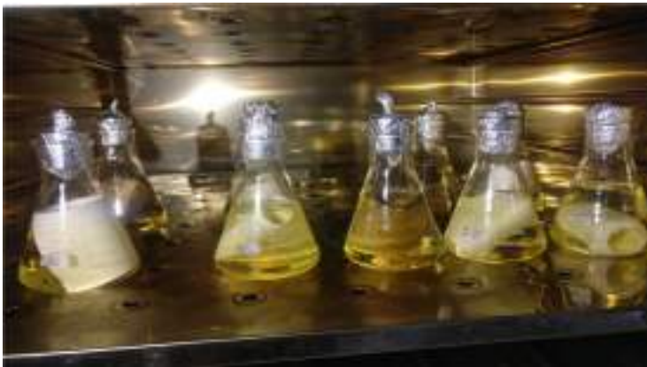
Fig. 1. Oil and paper insulation samples in Electric Oven.
