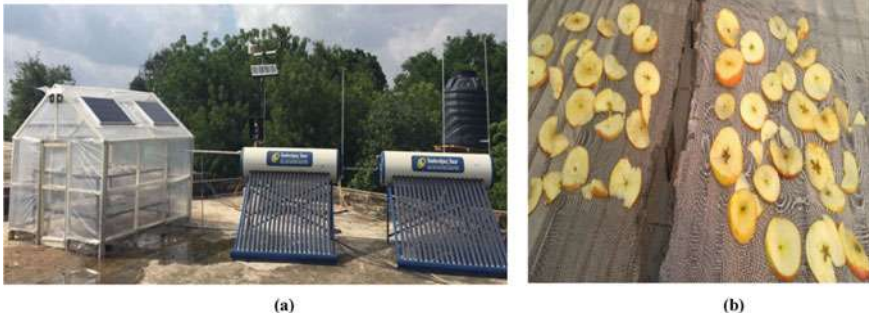
Fig. 2 Actual view of (a) installed hybrid solar drying system (b) drying tray loaded with the apple slices
