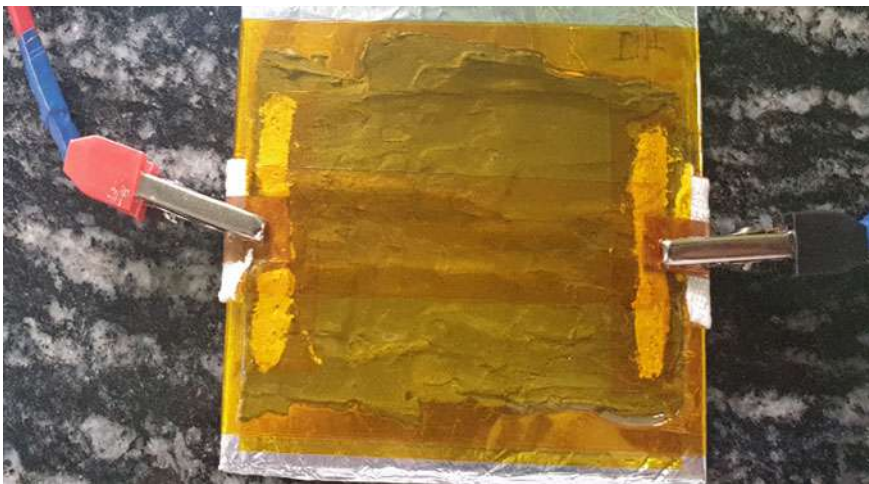
Fig. 2 Actual representation of the graphene layering
