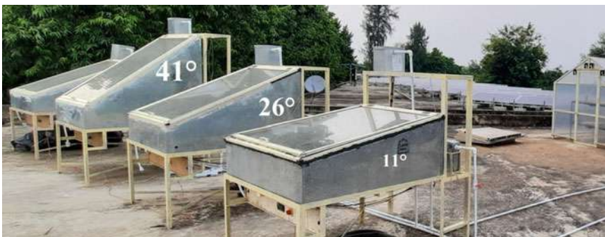
Fig. 1 Experimental setup with different tilt angles of the glass cover
