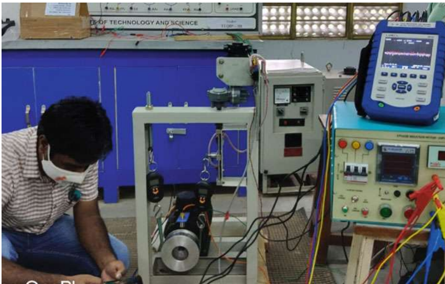
Fig. 3 Real-time data measurement from the motor under trial
