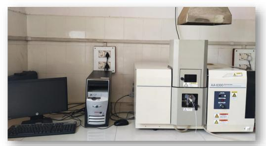
General Information-Make- Shimadzu Model- AA6300 Lamps Available -As, Cr, Cu, Fe, Hg, Na, Ni, Zn Fuel: Acetylene Oxidants: Air
