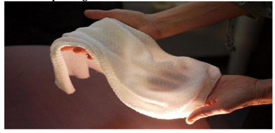
This new fabric being developed by University of Maryland scientists YuHuang Wang and Ouyang Min is the first textile to automatically change properties to trap or release heat depending on conditions. Despite decades of innovation in fabrics with high-tech thermal properties that keep marathon runners cool or alpine hikers warm, there has never been a material that changes its insulating properties in response to the environment.
