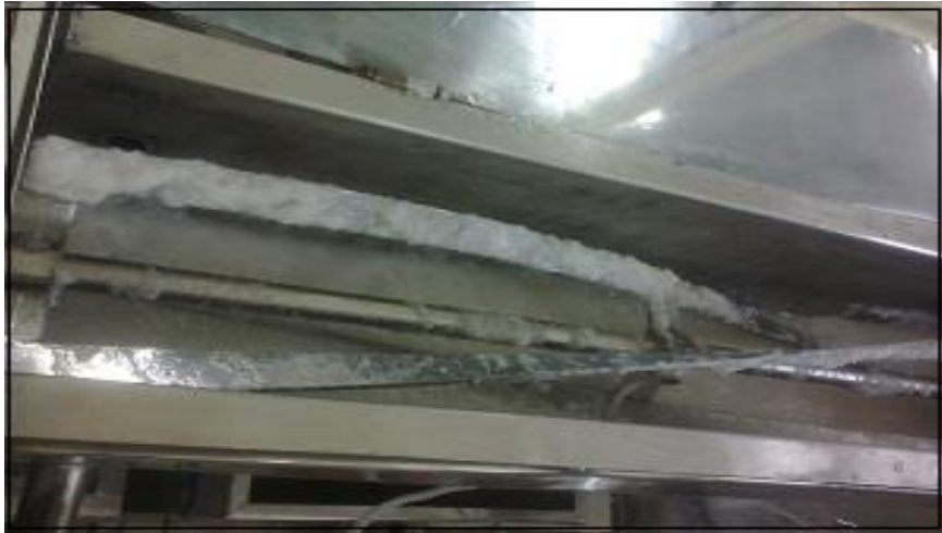
Fig.3. Crystal growth in crystallizer
