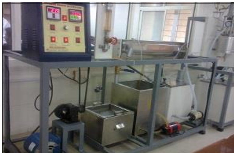
Fig.2. Pictorial view of Swenson Walker Crystallizer
