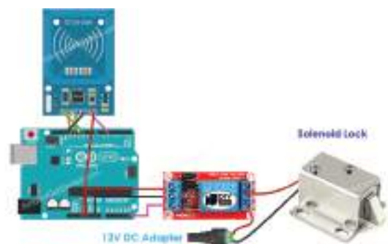
Fig. 1: Circuit Diagram of Arduino RFID Solenoid Lock for Home Security
