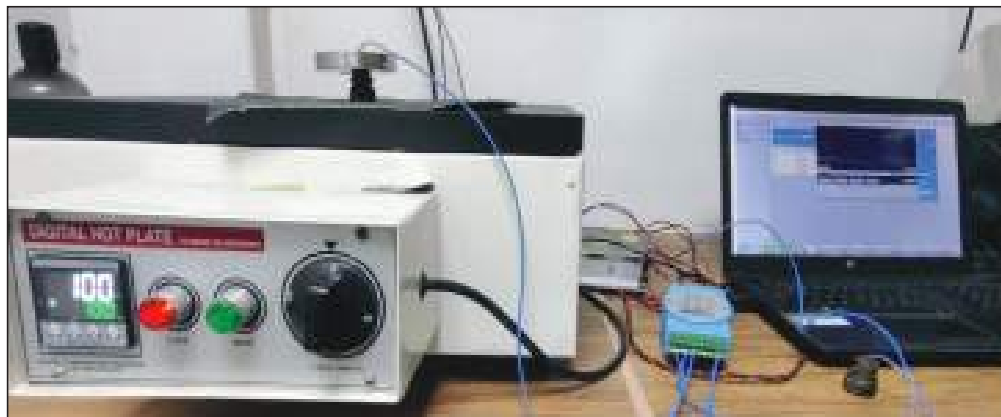
Fig. 6: Digital Hot Plate and Sensor Arrangement
