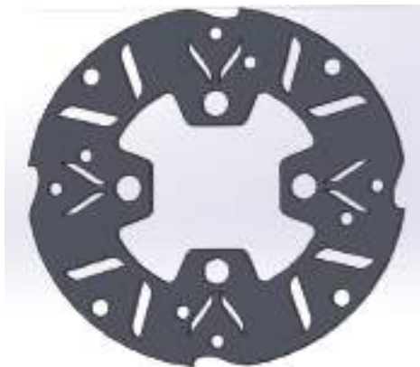
Fig 2.1: Design of Disc Rotor Thickness 5 mm Design in Solidworks
