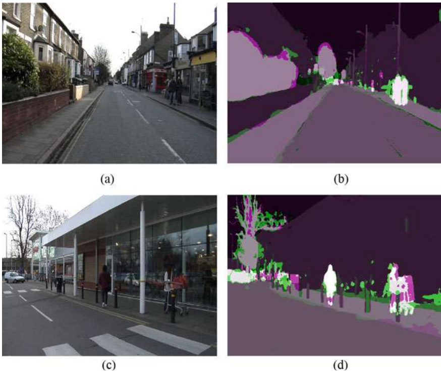
Fig. 8 The output of test data, where a , c are RGB frame from the CamVid dataset, b , d are corresponding segmented images
